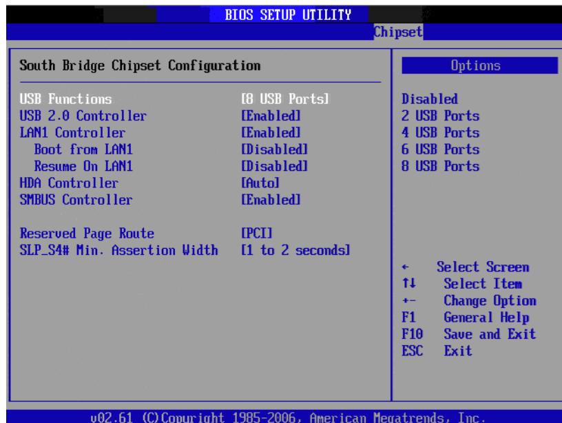
Figure 3.15 South Bridge Configuration
