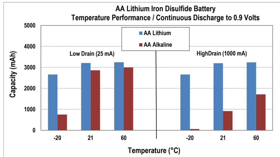
(Fig. 4) Temperature Effect on Performance versus Alkaline
