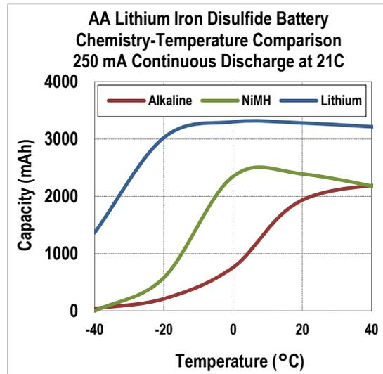
(Fig. 7) Impact of Temperature on AA Size Lithium, Alkaline and
