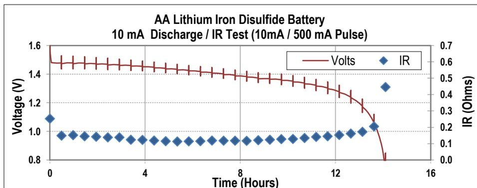
(Fig. 10) IR of a typical AA size lithium iron disulfide battery during discharge.
