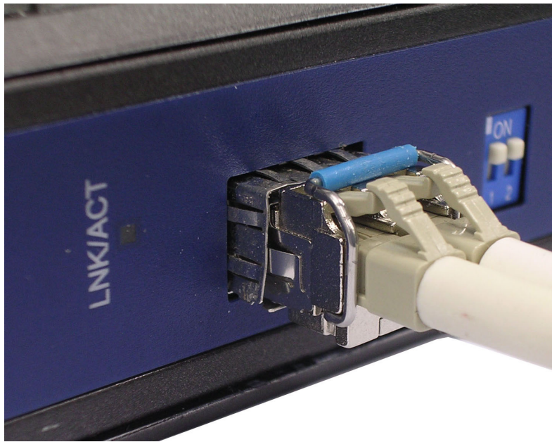
Figure 2.10: LC connector to the transceiver
