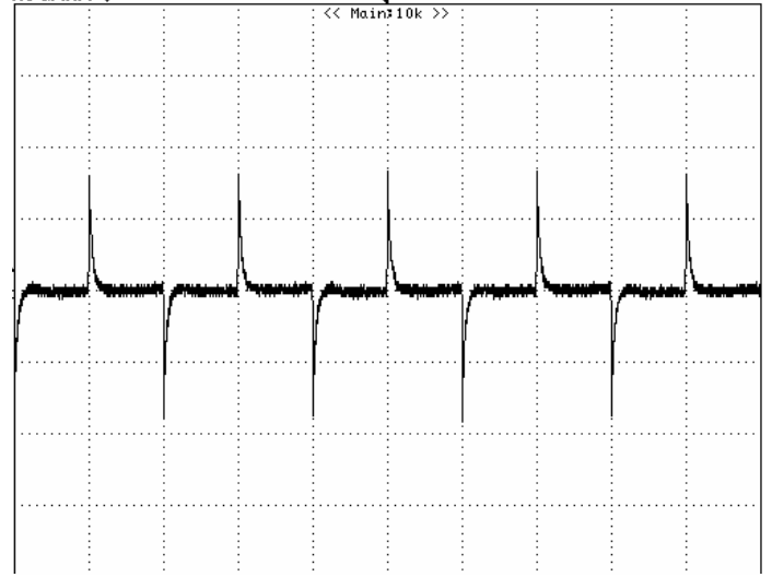
Figure 18: Typical transient response to step load change at 1A/\mu S from 100%~ 50%~100% of I_o , max at 12V_{in} , 2.5V_{out} ( C_{out} = 1\mu F ceramic, 47\mu F+10\mu F ceramic) CH1 : VOUT, 0.1V/div, 5mS/div
